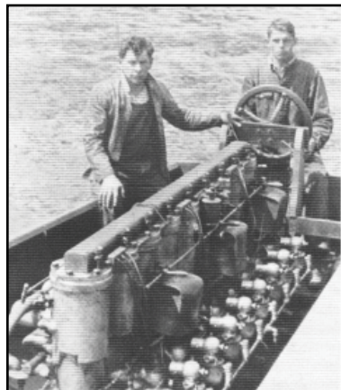
Johnny Wolff (left) and Oscar Peterson behind the 9-cylinder Smalley engine.
